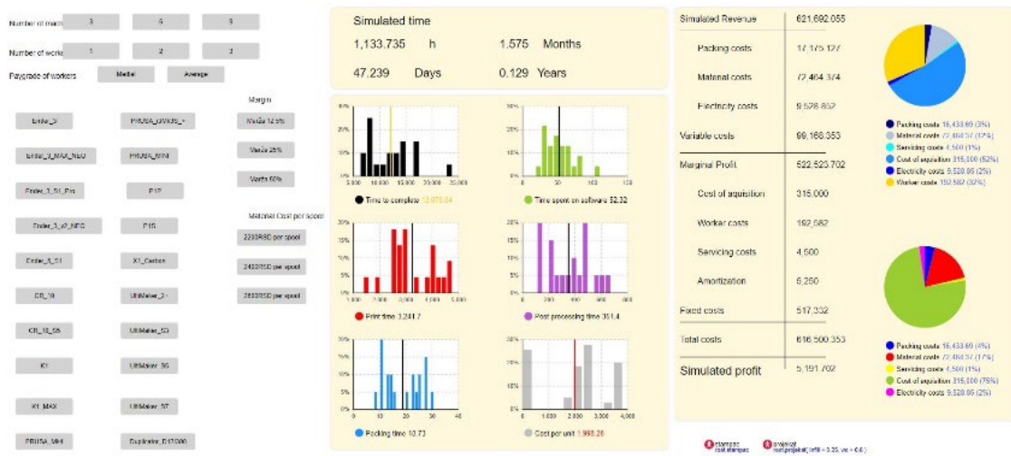
Figure 2: Break-even point for 9 Ender3 printers, where workers are paid the Median salary, margins are at 50% and the material used costs 2600 RSD/spool.
